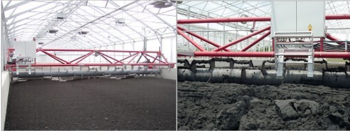
Figura B. The Wendewolf – Ther Heart of the Drying Plant.
